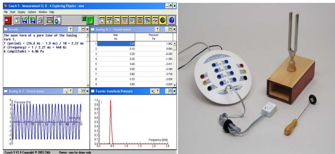
Figure 1: The Coach Lab panel, a microphone as sound sensor, a tuning fork, a typical graph of sound intensity versus time, and an intensity versus frequency plot.
