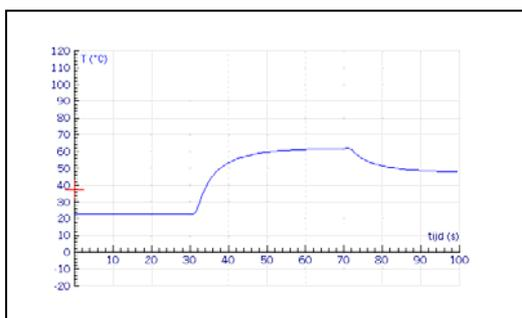
Figure 4: A graph of temperature versus time obtained by adding hot water to cold water and then adding cold water again.
